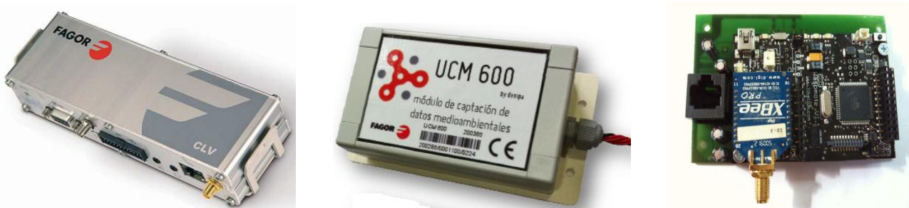
Figure 18: Detail of LPU, sensors and waspmote boards
