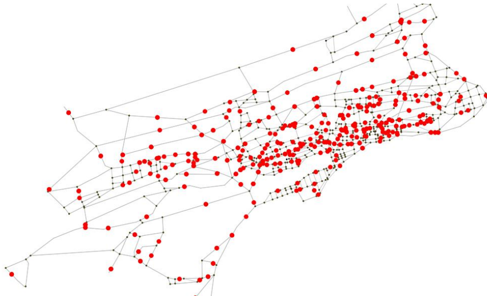
Figure 2: Sensor localization in Santander for capturing 100% of the traffic flow
