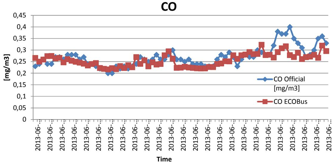
Figure 8: Comparison of official and EcoBus CO measurements
